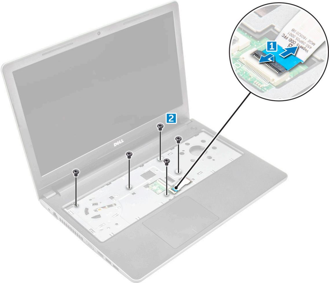
4 Remove the screws that secure the base cover to the computer
