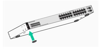
**Wall or Under-table Mounting:** To mount the 1820 24G, 1820 24G PoE+, 1820 24G PoE+, 1820 48G, and 1820 48G PoE+ switches:
