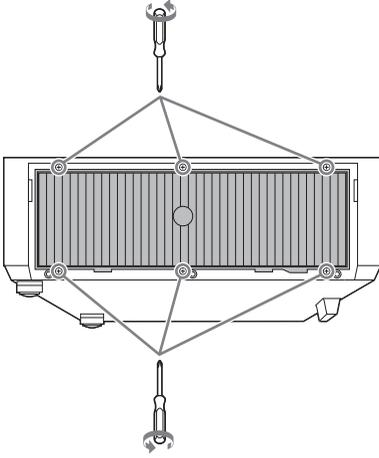
**7** Replace the air filter and attach the side cover.
