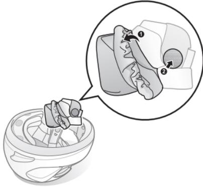
7. Attach the speaker and put the cover back on. Go through the same process for the other cheek pad.
