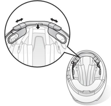
4. Peel off each cover of the hook and loop fasteners for speakers to expose the adhesive surface. Then, attach the fasteners to the ear pockets inside the helmet.
