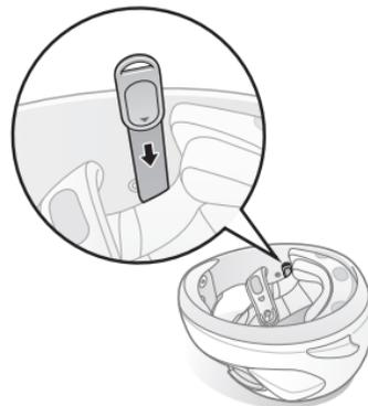
4. Peel off the cover of the adhesive tape of the control unit and attach it to the helmet.
