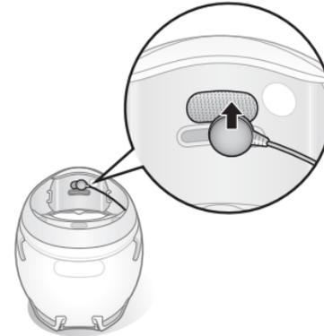
6. Remove the cover of the cheek pad, and attach the loop fastener for speakers on the corner of the ear pocket.
