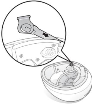
5. Align the left speaker with the left cheek pad base and insert the two clasps in the corresponding notches.
