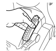
Remove the filter from the chamber.
