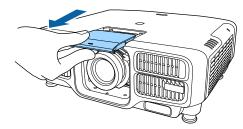
2 While holding the lens unit firmly, hold the lock lever and turn it counterclockwise to unlock the lens unit.
