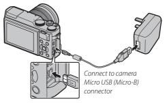
$\ensuremath{\mathbbm D}$  Be sure the connectors are in the correct orientation and then insert them fully.
