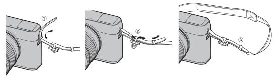
① To avoid dropping the camera, be sure the strap is correctly secured.
