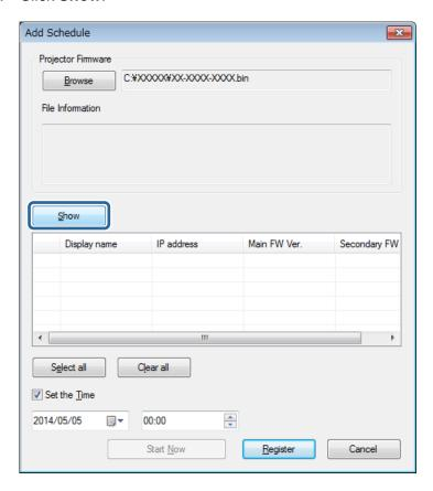
The firmware information is displayed in **File Information**, and then a list of the projectors that support the selected firmware is displayed.
