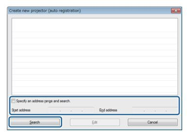
The application displays a list of network projectors that allow firmware updates or copying of menu settings using EasyMP Network Updater. If the projector you want is not displayed in the list, edit the projector list manually.
