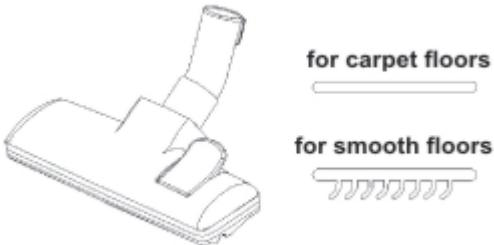
Clean carpets and wall-to-wall carpets without using the brush. Press the tip switch marked with the carpet symbol and the brush is raised.
