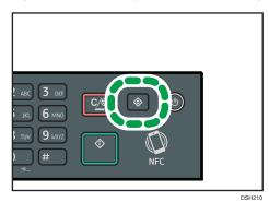
Otherwise, press the [◀] or [▶] key while "Ready" is displayed on the initial screen of the Copy, Scan, and Fax settings.
