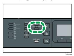
Press the [♠], [♥], [◄], or [▶] key to select the desired resolution, and then press the [OK] key.
