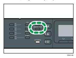
Press the [▲] or [▼] key to select the desired resolution setting, and then press the [OK] key.
