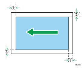
Margins when using exposure glass
