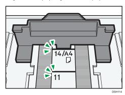
5. Check there are no gaps between the paper and the paper guides (both side and end paper guides).
