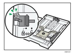
When using legal size paper, adjust the length to the position indicated by the mark " $\mathfrak{J}$ " in the tray.
