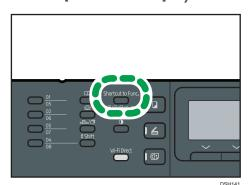
To make the [Shortcut to Func.] key enable ID card copy mode for the current job, [Shortcut to Function] under [Admin. Tools] must be set to [ID Card Copy Mode]. You can also assign the setting using Web Image Monitor.
