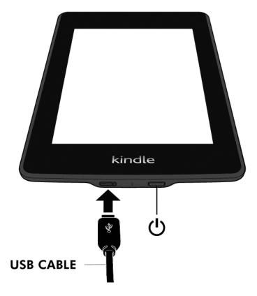
**Power button**: To turn your Kindle on, press the Power button located on the back. If you need to turn off your Kindle screen, press and hold the Power button for 7 seconds until the Power dialog box displays and then tap Screen Off.
