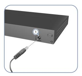
Figure 17: DC Power Cord and Power Socket
