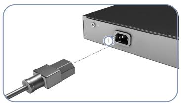
1) Plug the AC power cord into the socket on the rear of the switch.
