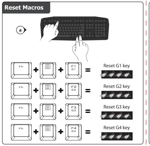
To reset an individual macro press FN + Menu/App + G1/G2/G3/G4 key. If the reset is executed correctly the LED in the top right corner of the keyboard will pulse 3 times.\* \*You can only reset a macro when Gaming Mode is activated.
