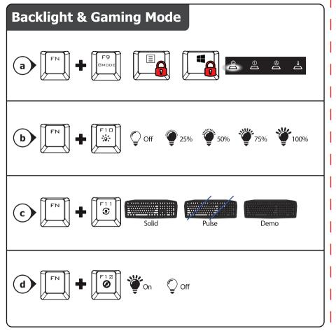
Gmode LED will lid up the upper right corner on the keyboard). When the gaming mode is active the Menu/App key and Windows key are locked
