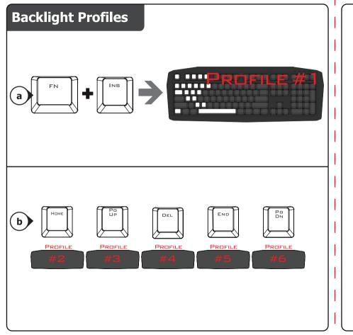
Backlight mode is activated, after that simply press FN + Insert for profile #1
