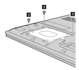
8 Remove the hard disk drive by gently pulling it in the direction of the arrow4. Take out the hard disk drive secured in a metal frame5.
