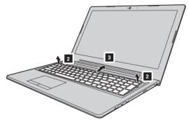
4 Lift up the keyboard 4 and detach the connector in the direction shown by the arrows 5 6.
