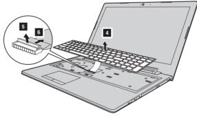
**6** Reinstall the new keyboard and tighten the screws.
