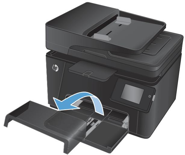
2. Load the paper into the tray. Make sure that the paper fits under the tabs and below the maximum-height indicators.
