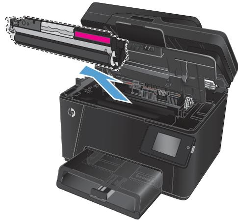
5. Remove the new toner cartridge from the bag. Place the used toner cartridge in the bag for recycling.
