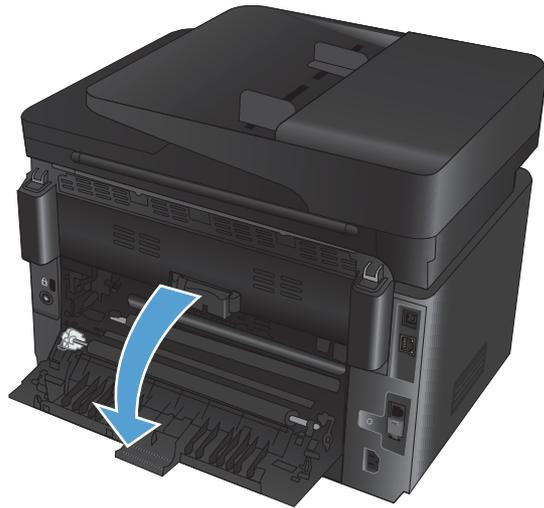
3. Remove any jammed paper. Use both hands to pull out the paper to avoid tearing.
