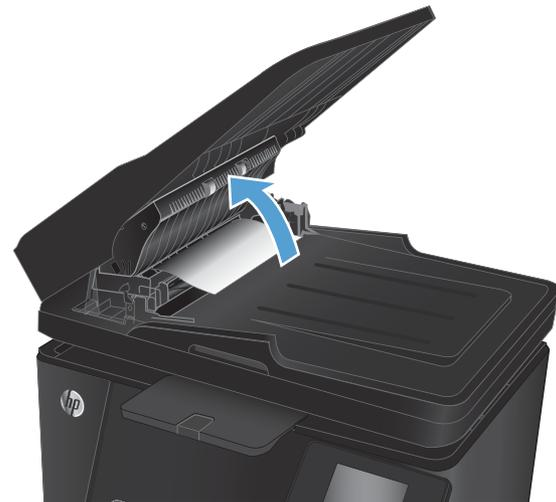
4. Remove any jammed paper. Use both hands to pull out the paper to avoid tearing.
