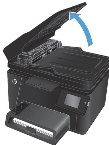
2. Use a moist, lint-free cloth to wipe both pickup rollers and the separation pad to remove dirt.
