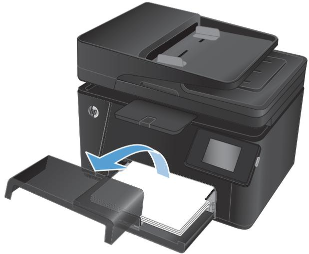
2. Remove the stack of paper from the input tray.
