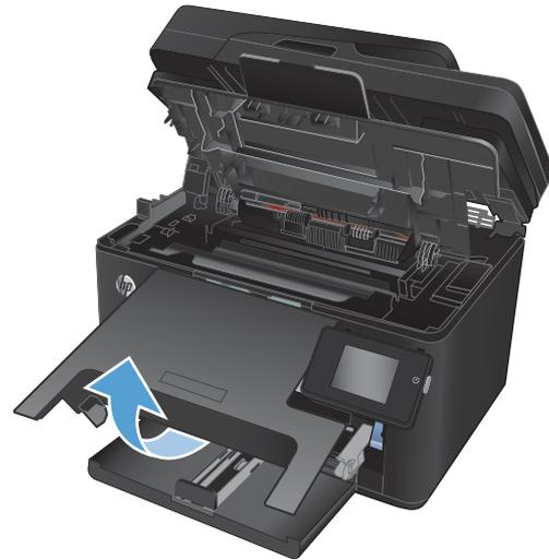
5. Lift the two levers that hold the imaging drum.
