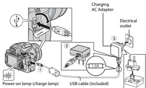
If a plug adapter\* is included with your camera, securely connect it to the Charging AC Adapter. Once the two are connected, attempting to forcibly remove the plug adapter could damage the product.
