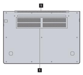
**1 Ventilation slots** Dissipate internal heat.
