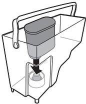
**16** Insert the AquaClean filter vertically onto the filter connection. Push the AquaClean filter to the lowest possible point. Make sure that the filter fits tightly and the seal is in the right position, to guarantee the best performance.
