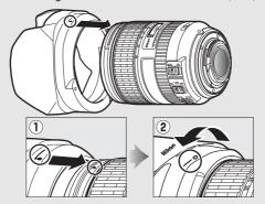
When attaching or removing the hood, hold it near the symbol on its base and avoid gripping it too tightly. Vignetting may occur if the hood is not correctly attached. The hood can be reversed and mounted on the lens when not in use.
