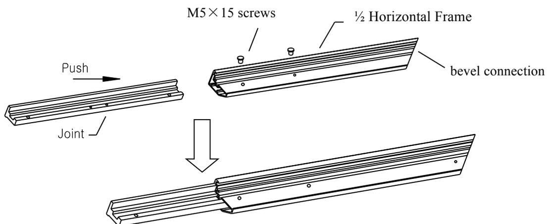
2. Insert the other 1/2 horizontal frame piece to the **center joint** connector and fasten it with two **M5x15 screws**. Repeat steps 1 and 2 for assembling the second horizontal frame.
