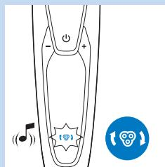
1 The shaving unit symbol lights up continuously, the arrows flash white and you hear a beep when you switch off the shaver.
