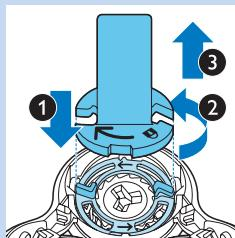
3 Place the retaining ring holder on the retaining ring (1), turn it anticlockwise (2) and lift it off the shaving head (3). Remove the retaining ring from the retaining ring holder and repeat this process for the other retaining rings.
