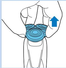
2 Pull the shaving head holder off the bottom part of the shaving unit.
