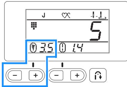
Each press of “-” makes the zigzag stitch narrower.
