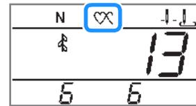
→ If pressed again, it turns to (single sewing), and machine will stop sewing at end of combined patterns.
