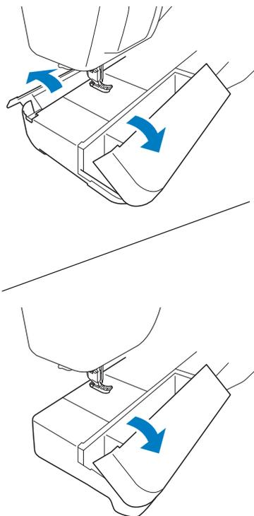
A presser foot accessory tray is stored in the accessory compartment of the flat bed attachment.
