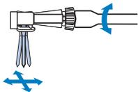
**6** With the flat side of the needle toward the rear of the machine, insert the needle until it touches the needle stopper.
