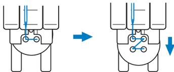
**7** Turn the handwheel toward you (counterclockwise) to check that the needle correctly goes into the two holes of the button.
