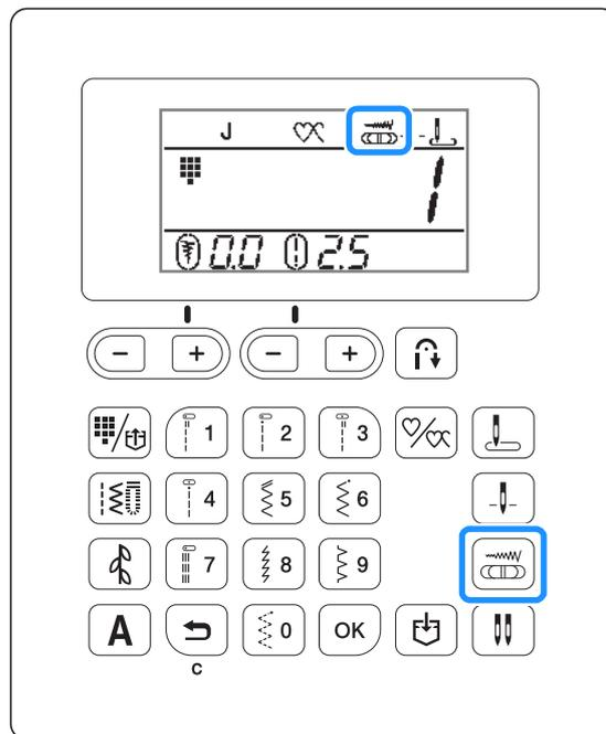
→ The machine is now set so that the stitch width can be controlled with the sewing speed controller.
