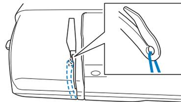
**11 Slide the thread behind the needle bar thread guide.**
