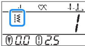
2 Enter the number of the desired stitch using numeric keys, and then press
