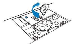
Turn the handwheel to check that the feed dogs move smoothly and do not contact the edges of the slots in the needle plate.
