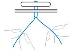
**10** When you are finished attaching the button, slide the feed dog position switch, to
