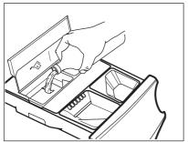
Gently pour only liquid softener in the AutoDose fabric softener tank . Fill up to the maximum indicated level MAX
