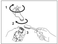
Remove the inlet hose from the appliance by loosening the ring nut.
