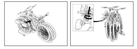
7) Place the light panel at the end of the bended rods, tighten the screws.
