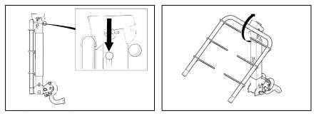
5) Press the peg in the direction of arrow, set the bended rods into horizontal position, check the peg fits correctly.
