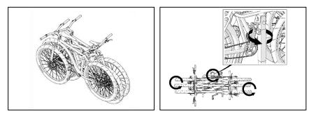
6) Mount the bikes inversely (seat to handlebars), tie a pedal of the first bike to the bike carrier, tie remaining bikes with straps together.
