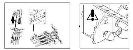
Push your carrier towards the car, lift the control ball and tilt slowly to position 1 or 2.
