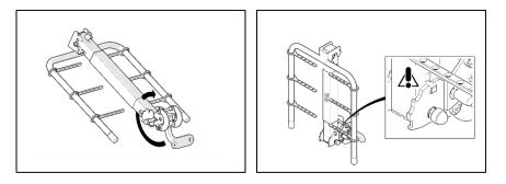
4) Hold the control ball and lift the carrier into driving position. Check the square bar fits as illustrated in the picture.
