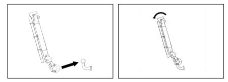
1) Place the bike carrier on the tow bar (lower "jaw" and upper "bowl" encircle the tow bar), push the body of the carrier in the direction of the arrow.
