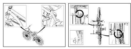
5) Hang up the bike on the bike carrier as illustrated (on lower frame and below seatpost), tighten the frame with rubber belts by the screw heads located at the bottom of the bended rods.
