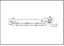
Push the locking peg in your direction (as arrow shows) and simultaneously tilt up upwards the body of the bike rack.
