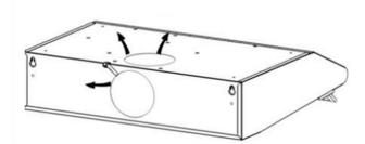
For indoor air ventilation, install the carbon filter, turn on the cooker hood, then the air will be vented inside.
