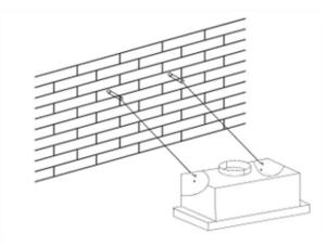
Fix the cooker hood with safety screw. The two safety vents are position on the back casing, with diameter of 6mm. Put the one way valve onto the cooker hood.
