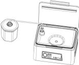
2. Touch the "Vacuum Sealing" button two second to to start vacuuming— *Fig.* 2. To ensure there is no air leaking between the cover and the canister, use your hand to push down the cover at the beginning of the vacuuming work. The machine will stop automatically when enough vacuum pressure is achieved.
