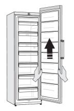
Remove the door from the bottom hinge by carefully lifting the door straight up. Lay the door onto a smooth surface.
