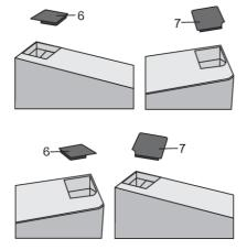
Remove the cap (6) from the left side of the door. Then, remove the cap (7) from the right side of the door. Place the cap (7) on the left side of the door and place the cap (6) on the right side of the door.
