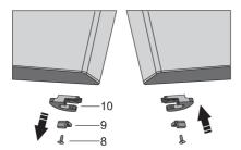
Undo the screw (8) and remove the door retainer (10) and the door stop (9). Then, use a screw (8) to install the door retainer supplied in the bag, and the door stop (9). Keep the door retainer (10) in case you need it later.
