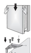
Place the door on the bottom hinge and use the screws (2) to attach the top hinge (3). Hold the door in place while positioning it. 11.
