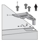
Undo the screws (2) and remove the hinge (3). Hold the door while doing this to prevent it from falling.
