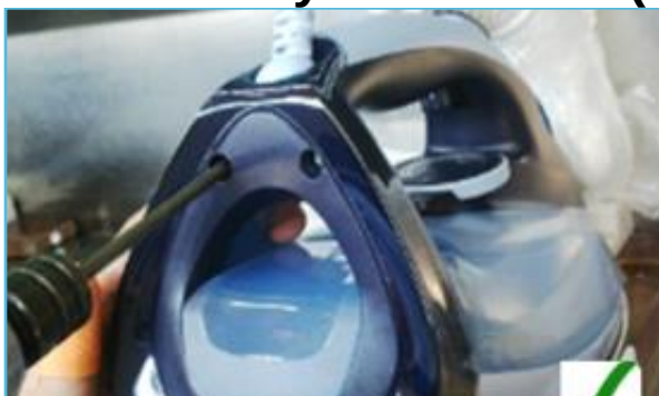
27. Tighten BACKPLATE 1 to WATER TANK ASSY 7 with 2x Screw A1
