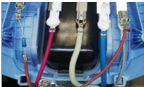
7. Apply Heat Sink Paste onto pink terminal of ASO 1 and blue terminal of MAINSCORD 6 to Frame Connector
