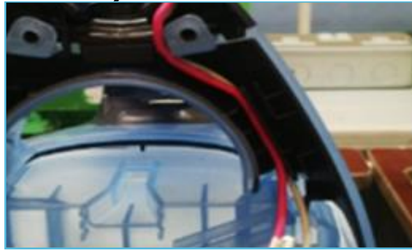
10. Dress grey and pink wires onto slot on the right side of half-ring plate
