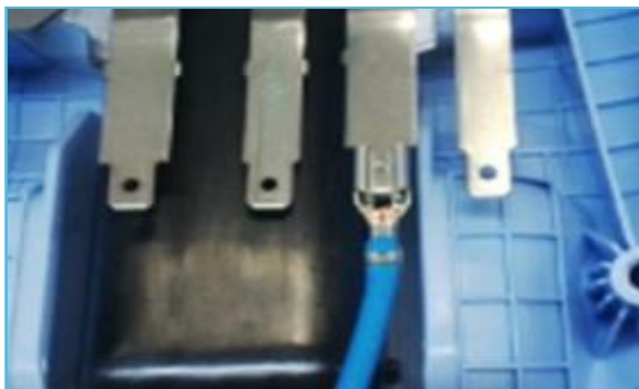
2. Connect blue wire of MAINSCORD 6 to 'N' Frame Connector (second from the right)
