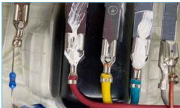
17. Remove the Heat Sink Paste from the connectors with clean cloth. Press the tab of Quick Connector on MAINSCORD and pull it out from Frame Connector.
