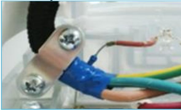
22. Assemble Clamping Plate, assemble & fasten 2x Screw A2
