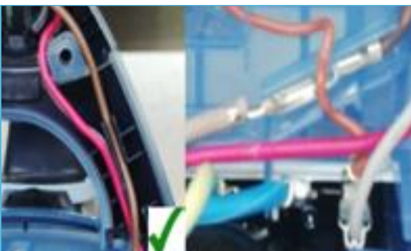
20. Dress brown wire onto slot on the right side of half-ring plate, and also dress the connection into slot on Tank Top
