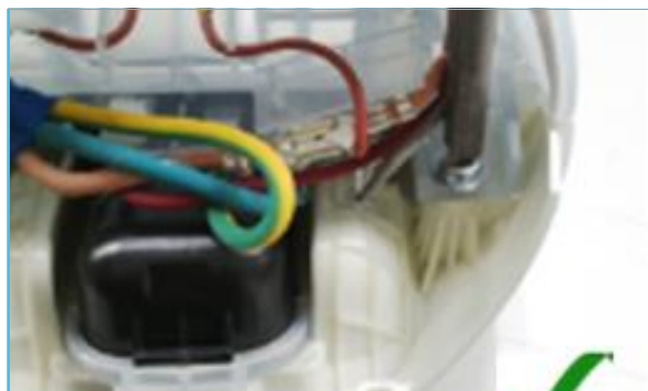
14. Assemble and fasten 2x Screw A3 at rear of WATER TANK ASSY 7 to Cover
