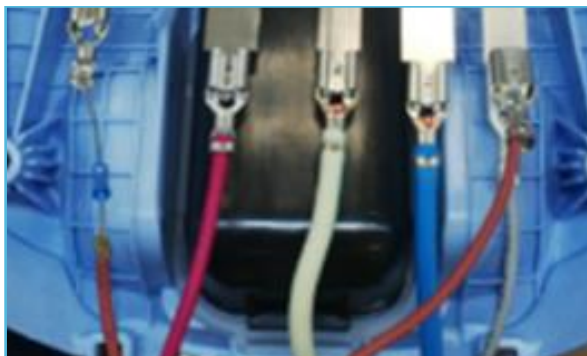
6. Connect the brown wire without resistor of Lamp Assy 9 to piggy-back connector of the ASO 1 grey wire
