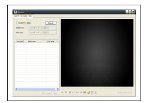
Attention: press 2x on the file you want to watch. It opens the window (see left). You press with right mouse at the display of the window and after this you can use the button displayed.
