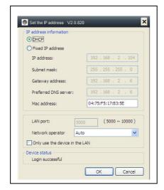
The default setting is camera use DHCP. Camera auto gets IP address from network router.
