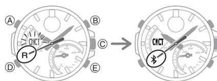
3. Perform the operation shown on the phone screen to correct hand alignment.
