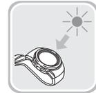
While you are wearing the watch, make sure that its face (solar panel) is not blocked from light by the sleeve of your clothing. Power generation efficiency is reduced even when the face of the watch is blocked only partially.
