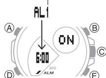
3. Press (A) to turn off the displayed alarm or the hourly time signal.
