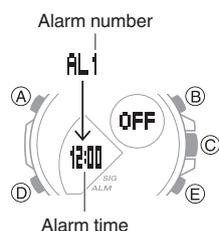
3. Hold down (A) for at least two seconds. Release the button when the hours digits start to flash.
