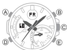
2. Hold down (A) for at least two seconds. Release the button when the name of the currently selected Home City appears on the display.
