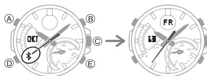
2. If the watch is in any mode besides the Timekeeping Mode, hold down (D) for at least two seconds to enter the Timekeeping Mode.
