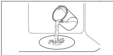
The maximum capacity of the cavity embossment is 250 ml. Do not refill the cavity embossment during cooking or when the appliance is hot.
