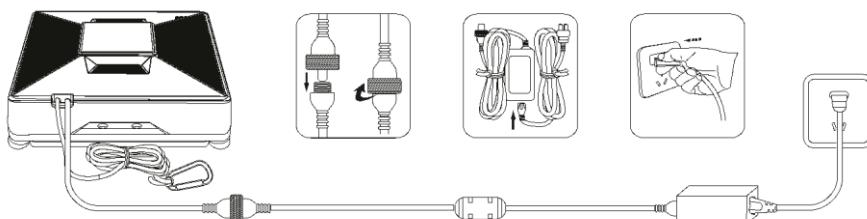
Install a safety cable in a suitable location and adjust its length to secure the device against falling. Make sure that the length of the cable or rope does not restrict the movement of the device on the window.
