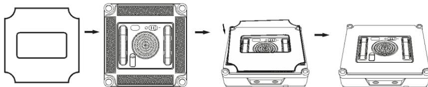
Open the silicone cap of the water tank (7) and pour clean water into the tank using the plastic container provided. Do not overfill the water tank (80 % full is sufficient) to maintain stable air pressure.
