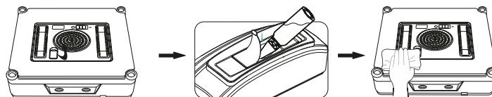
Use only clean distilled water to prevent limescale buildup and clogging of the water jets. Do not add any cleaning agents that may cause foaming, streaking, or clogging of the water jets. If the condition of the window requires it, you can use a small amount of a good quality, non-foaming, low-alcohol window cleaner to moisten the cleaning cloth or window surface.
