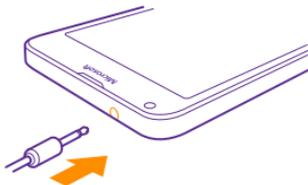
Do not connect to products that create an output signal, as this may damage the device. Do not connect any voltage source to the audio connector. If you connect an external device or headset, other than those approved for use with this device, to the audio connector, pay special attention to volume levels.
