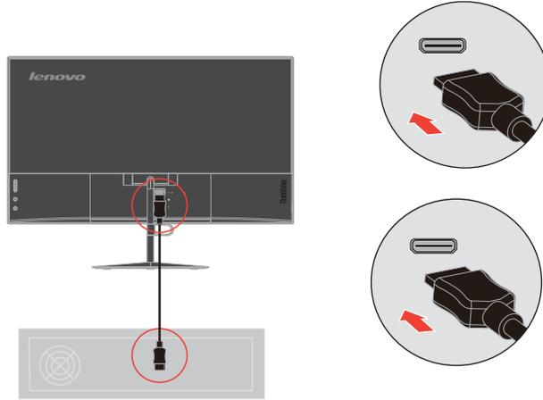
5. Insert the Adapter cord into the monitor, then plug the monitor power cord and the computer cord into grounded electrical outlets.
