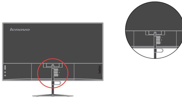
3. Connect one end of the DP cable to the DP connector on the back of the computer, and the other end to the DP connector on the monitor.
