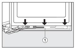
Prise open panel ① from the SoftClose mechanism: Remove the panel carefully from the top. Take care not to damage the door seal.
