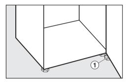
■ The foot ③ should **definitely** be unscrewed until it rests on the floor. Then turn it a further 90°.
