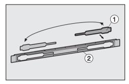
Remove cover ① from panel ②, rotate it by 180° and refit it on the other side.
