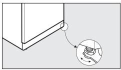
Align the front feet using a flat spanner.
