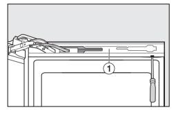
Prise open panel ① from the SoftClose mechanism: Insert a flat-bladed screwdriver into the gaps from below and ease it off bit by bit.
