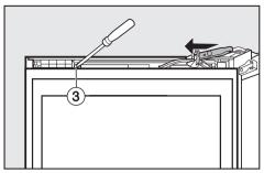
Tighten the spacer and the SoftClose mechanism with screw 3.
