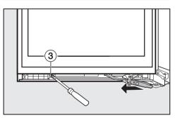
■ Tighten the spacer and the SoftClose mechanism with screw ③.
