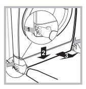
3. remove the cover panel on the lower front part of the washing machine (see figure).
