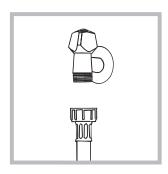
1. Connect the supply pipe by screwing it to a cold water tap using a ¾ gas threaded connection (see figure). Before performing the connection, allow the water to run freely until it is perfectly clear.
