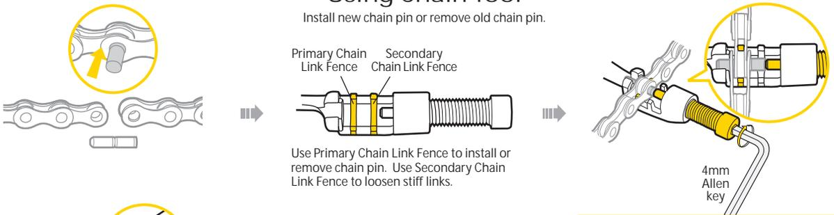
Use Primary Chain Link Fence to install or remove chain pin. Use Secondary Chain Link Fence to loosen stiff links.
