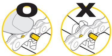
When pressing in the chain pin, push down on the top of the chain to keep it fully engaged in the chain tool cradle. Make sure the press pin of the chain tool is centered against the chain pin.
