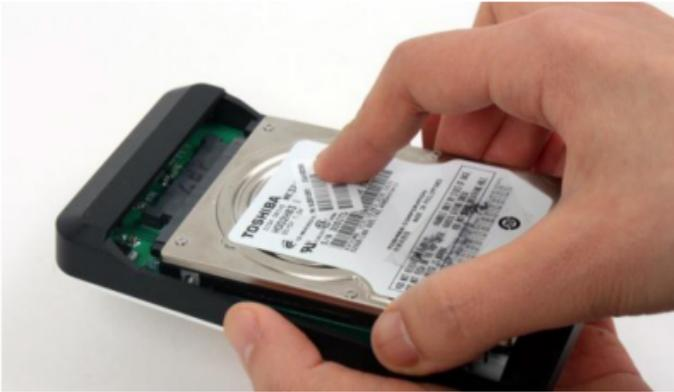
③Close the back panel by pushing up according to the arrow direction. ZM-SHE350 supports screw-less HDD installation.
