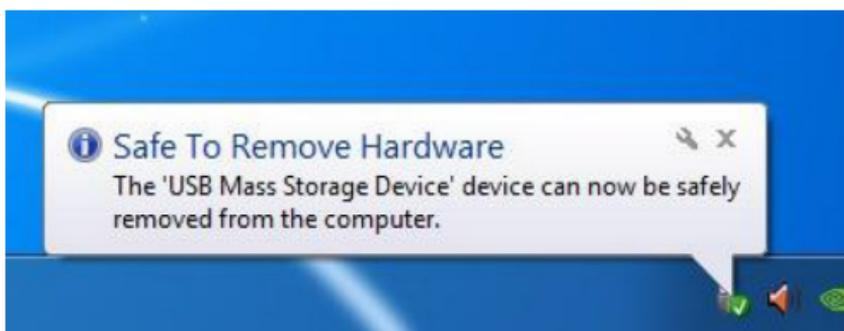
ZM-SHE350 supports smart MOUNT and UN-MOUNT feature to make simple, convenient and safe hardware removal. Press "MENU" button over 2 seconds, then HDD is automatically disconnected. It works like [Safely Remove Hardware]. \* To run this function, there should be no data transfer between PC and ZM-SHE350 at that time.
