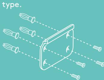
2 Attach the camera to the bracket.
