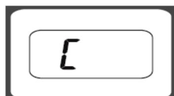
Display shows „C“ when you step off the scale, means this reading with error. Please re-test.
