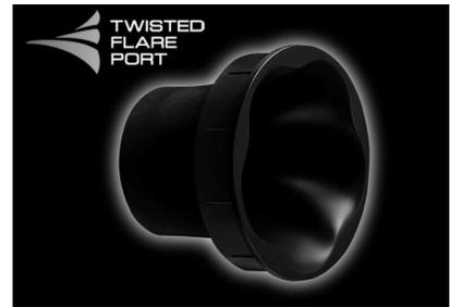
The Twisted Flare Port developed by Yamaha changes the way in which the port widens toward its end, and also adds a “twist” to suppress airflow turbulence at each end of the port and thus prevent noise from occurring. This eliminates the “muddy sound” and “wind noise” that until now have been characteristic of bass reflex speakers, allowing bass to be reproduced clearly.
