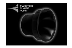
The Twisted Flare Port developed by Yamaha changes the way in which the port widens toward its end, and also adds a "twist" to suppress airflow turbulence at each end of the port and thus prevent noise from occurring.
