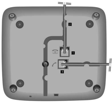
Connect the telephone connector (1) to the main telephone socket. Use the telephone cable supplied.
