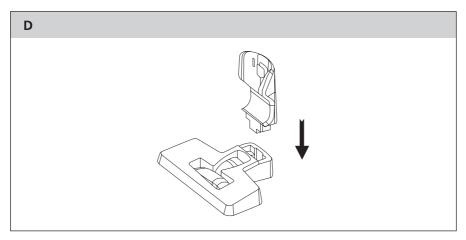
When disassembling the charging base A<sup>®</sup>, it is necessary to first release the clip on the underside
