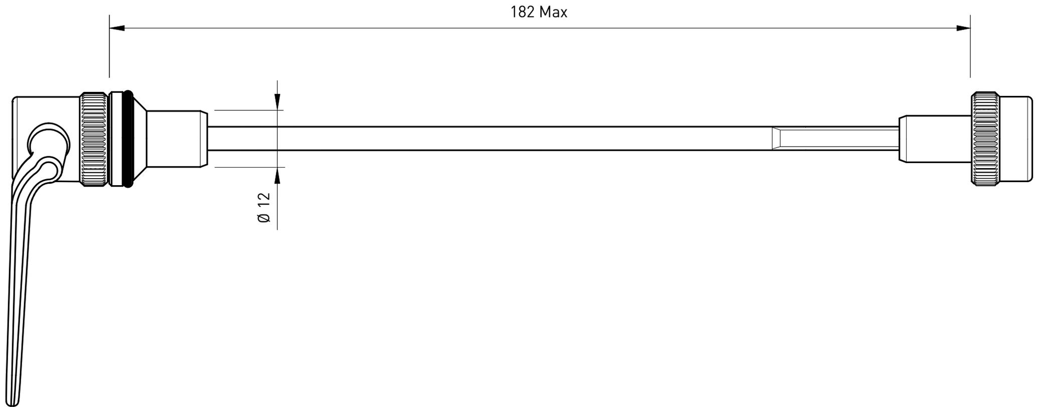
All sizes are shown in millimeters (mm)
