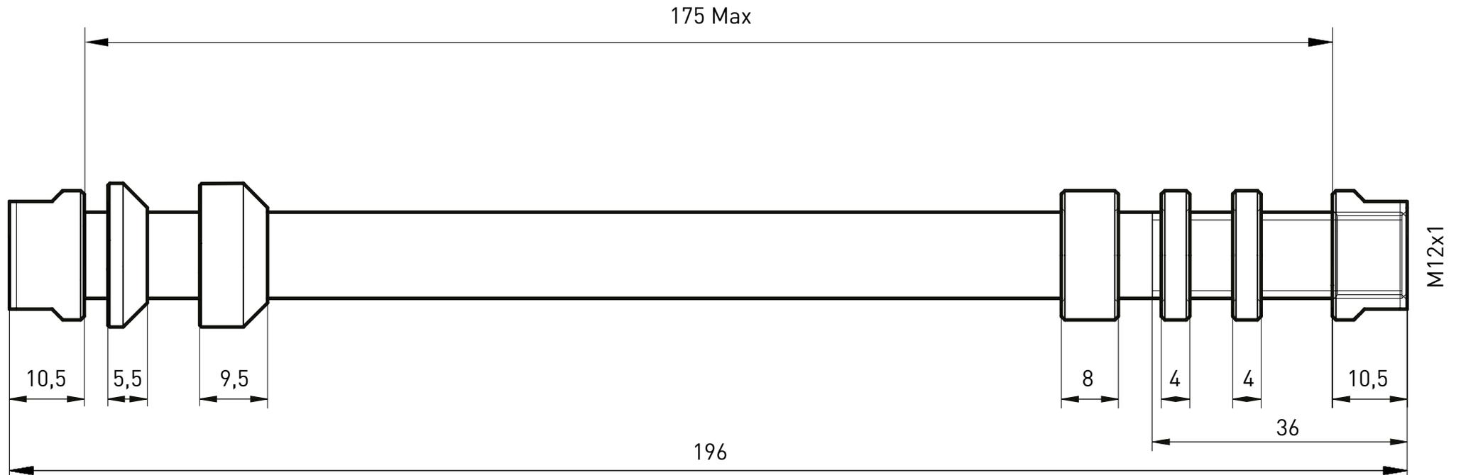
All sizes are shown in millimeters (mm)
