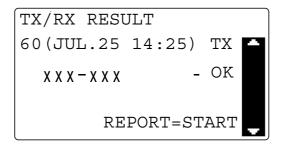
If **Network Card NC-504** or **Image Controller IC-209** is installed on this machine, NTP server can be set. Contents of displayed communication results differ depending on whether or not the NTP server has been specified.
