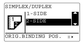
→ When you select [2-SIDE] and press ▶, you can specify the binding direction of the original. Select [LEFT] or [TOP], then press OK.
