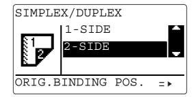
→ When you select [2-SIDE] and press ▶, you can specify the binding direction of the original. Select [LEFT] or [TOP], then press OK.
