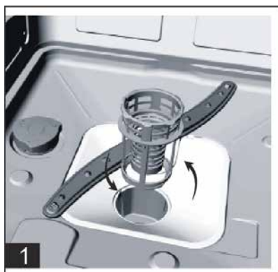
Korak 1: Filter zasučite proti smeri urnega kazalca in ga izvalcite.
