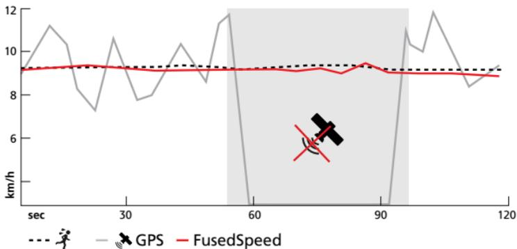
FusedSpeed benefits you the most when you need highly reactive speed readings during training, for example, when running on uneven terrain or during interval training. If you temporarily lose the GPS signal, for example, Suunto Ambit3 Peak is able to continue showing accurate speed readings with the help of the GPS calibrated accelerometer.
