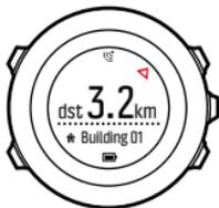
While moving (>4 km/h), the watch shows you the direction to the POI (or waypoint if navigating a route) based on GPS.
