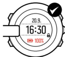
Fully charging an empty battery takes about 2-3 hours. Buttons are locked while the USB cable is attached and connected to a computer.
