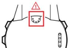
**⚠ CAUTION:** *Keep the area around the sensor free of dirt and sand. Never insert any objects into the sensor openings.*
