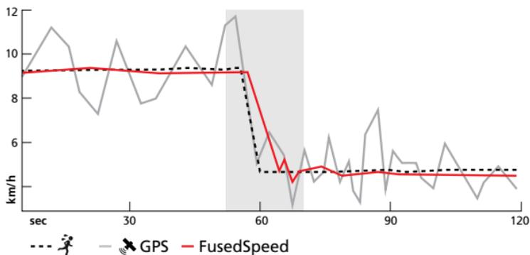
**TIP:** To get the most accurate readings with FusedSpeed, only glance shortly at the watch when needed. Holding the watch in front of you without moving it reduces the accuracy.
