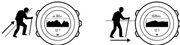
It is not possible to measure weather and altitude changes at the same time, as both cause a change in the surrounding air pressure. Suunto Ambit3 Peak senses vertical movement and switches to measuring altitude, when needed. When altitude is shown, it is updated with a maximum delay of 10 seconds.
