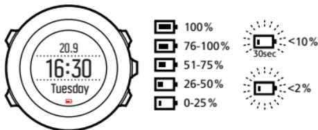
Charge the battery by attaching it to your computer with the supplied USB cable, or charge with a USB-compatible wall charger. It takes approximately 2-3 hours to fully charge an empty battery.
