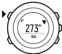
The compass switches to power saving mode after one minute. Reactivate it with [Start Stop].
