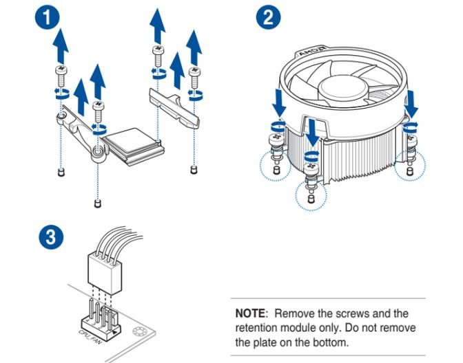
**NOTE:** Remove the screws and the retention module only. Do not remove the plate on the bottom.
